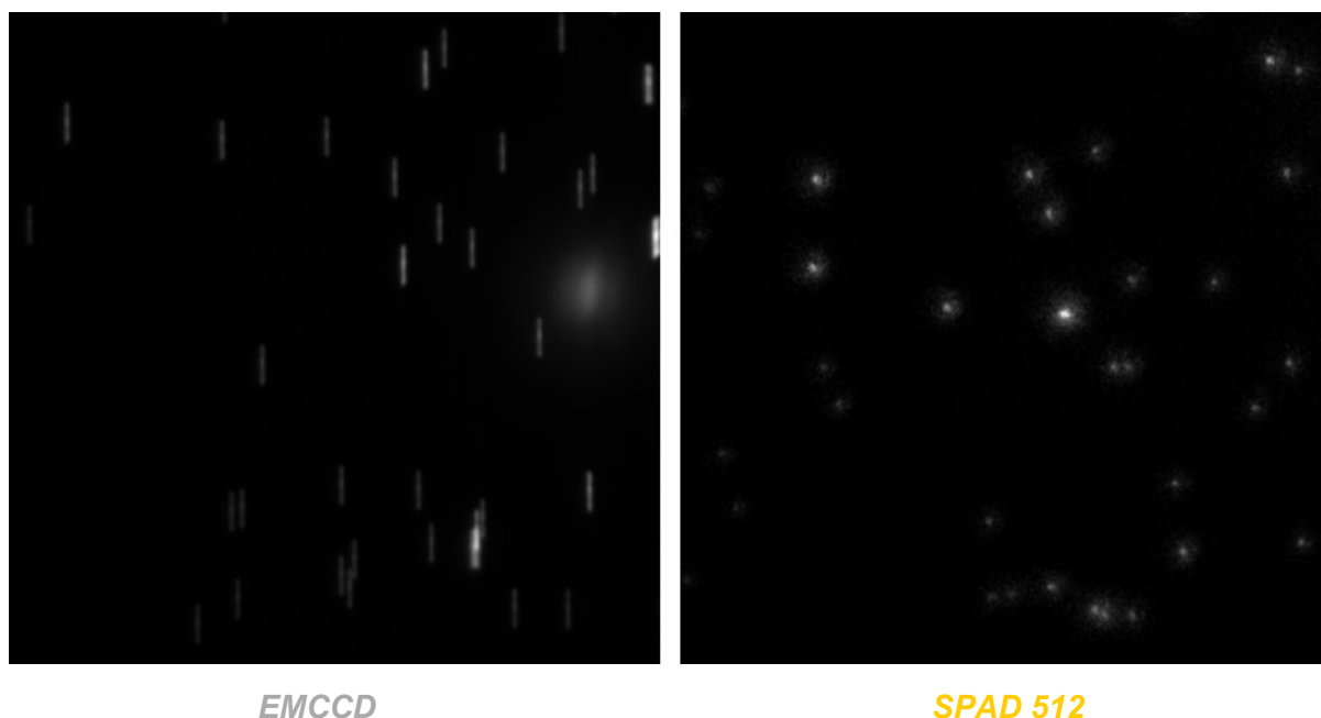
Figure (2): Images of moving fluorescent beads with EMCCD camera (56 fps) and SPAD 512 (1'600 fps).
